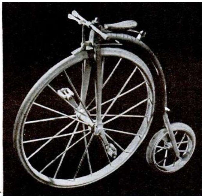
Special-prize winner A. A. Avritt's entry was this nostalgic replica of an old-fashioned big-wheeler. Dowels were used for everything except the wheel rims, which were turned from a piece of flat stock
